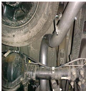
**7.** Install over axle tail pipe #C into muffler 1 1/2"-2". Use clamp #F to secure pipe to muffler. Do not tighten.
