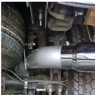
**8.** Slide exit pipe #D onto over axle tail pipe. Insert welded hanger into rubber grommet. Use clamp #F to secure pipes together. Do not tighten. Rotate pipe until level.
