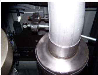
**4.** Slide muffler #B onto head pipe #A 1 1/2"-2". Use a jack stand to support the muffler. Use band clamp #G to secure the muffler to the head pipe, slide hanger on band clamp into rubber grommet. Do not tighten.
