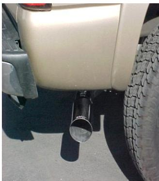
**11.** Install stainless steel tips. Clamp down. When you have everything in place, firmly tighten all bolts and clamps down securely. Use stainless steel cleaner and a Scotch Brite pad weekly to prevent tip from discoloration. Inspect all fasteners after 25-50 miles of operation and re-tighten as necessary.
